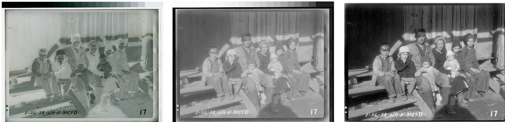
On the left is an image of a historic black-and-white film negative that was scanned in color with a positive tonal orientation (the digital image appears the same as the original negative), this represents a reasonably accurate rendition of the original negative. The middle grayscale image shows a direct inversion of the tones, and as shown here, often a direct inversion of a scan of a negative will not produce a well-rendered photographic image. The image on the right illustrates an adjusted version where the brightness and contrast of the image has been optimized (using "Curves" and "Levels" in Adobe Photoshop software) to produce a reasonable representation of the photographic image, these adjustments are very similar to how a photographer prints a negative in the darkroom. [photograph- NRCA-142-INFO01-3169D, RG 142 Records of the TVA, NARA – Southeast Region (Atlanta)]
